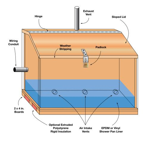
Even if a box can be less than 48 inches long, a larger enclosure may be justified. A small system that uses golf-cart batteries may some day be upgraded to L16s or industrial 2 V cells. A golf-cart battery is about  $10^{1}/2$  inches long; an L16 is about  $12^{1}/4$  inches. So upsizing the box initially to fit future battery possibilities may save money in the long run.
